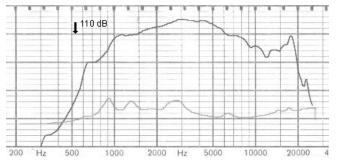
BMS 4554, 60° x 40° elliptical waveguide, SPL 10W / 1m
