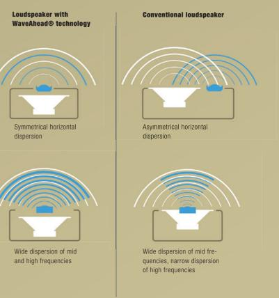
The coaxial arrangement of the WaveAhead® technology solves the interference issues of conventional loudpseakers and allows for a wide and even sound dispersion. With this unique setup you get the best of both worlds, an extra large sound coverage and a very compact design.
