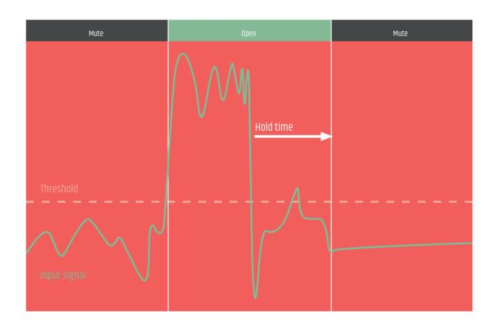
The U500 receiver's noise gate provides a choice of AUTOMATIC or MANUAL modes of threshold and hold time setting.
